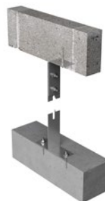
Base fixed using M12 FBN II Anchor into concrete slab.
