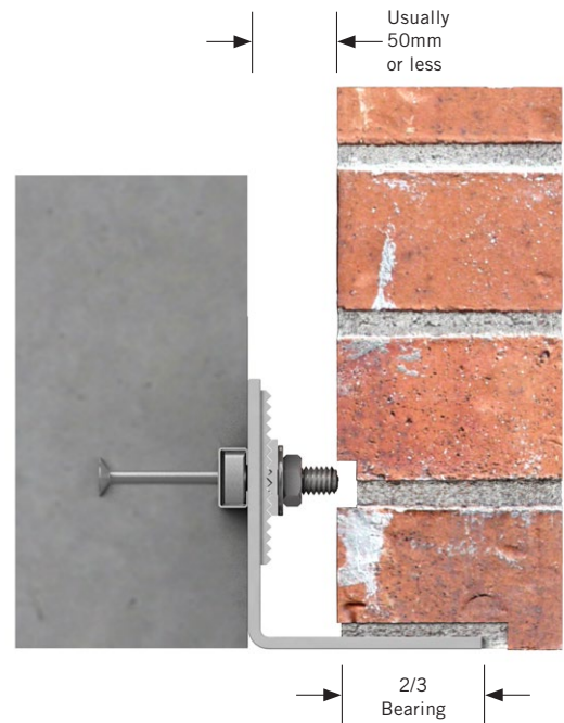
Typical Support Angle Condition
